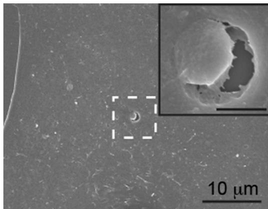
To create the nanoblade's "cat door" opening, researchers angle the micropipette tip on the cell's surface, fashioning a flap that the cell can easily repair. Reproduced with permission from ref. 3.
