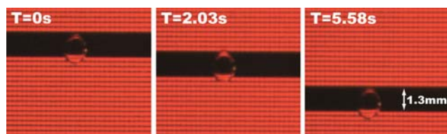
Fig. 9 Optical actuation of a droplet in a SCOEW device directly positioned on top of the LCD display of a personal computer.
